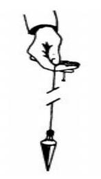
The importance of having both ends of the chain at the same elevation when measuring a horizontal distance cannot be over emphasized. One of the most common errors in chaining is failure to hold both ends of the chain at the same level.
