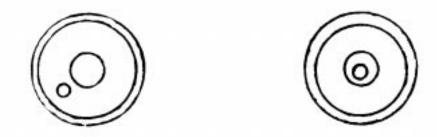
A right angle prism, or mirror, is usually mounted over the circular bubble vial to allow the instrument person to observe the bubble from his normal operating position, The bubble need only be inside the circle etched in the center of the circular vial for the instrument to operate satisfactorily. Thus the instrument person does not have to go through the time consuming procedure of precisely leveling the telescope tube as required for the Wye and Dumpy Levels.
