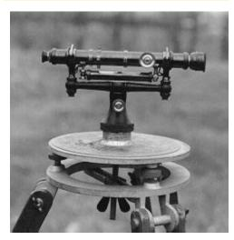
There are three types of levels used in construction surveying: The Wye Level, the Dumpy Level, and the Self-Leveling Level. All are designed to project a level line of sight when used properly.
